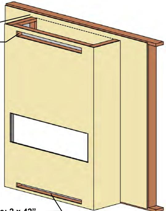
Lower Vent Slot (MIN **84** Sq. In.) is REQUIRED for ALL Installations. Example: 2 x 42"
