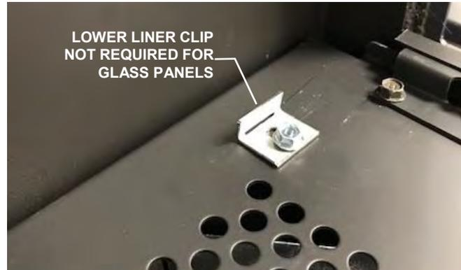
**STEP THREE:** Install one Glass Back Liner at each end of the firebox. Attach with 1 DT Screw on top corners and 2 at bottom.
