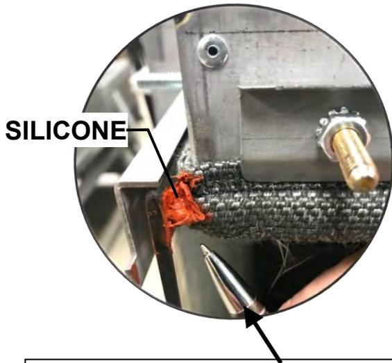
**⚠ IMPORTANT:** Each corner must have a dab of high-temp silicone placed between the ball of the gasket and the corner glass. This will fully seal the firebox corners.
