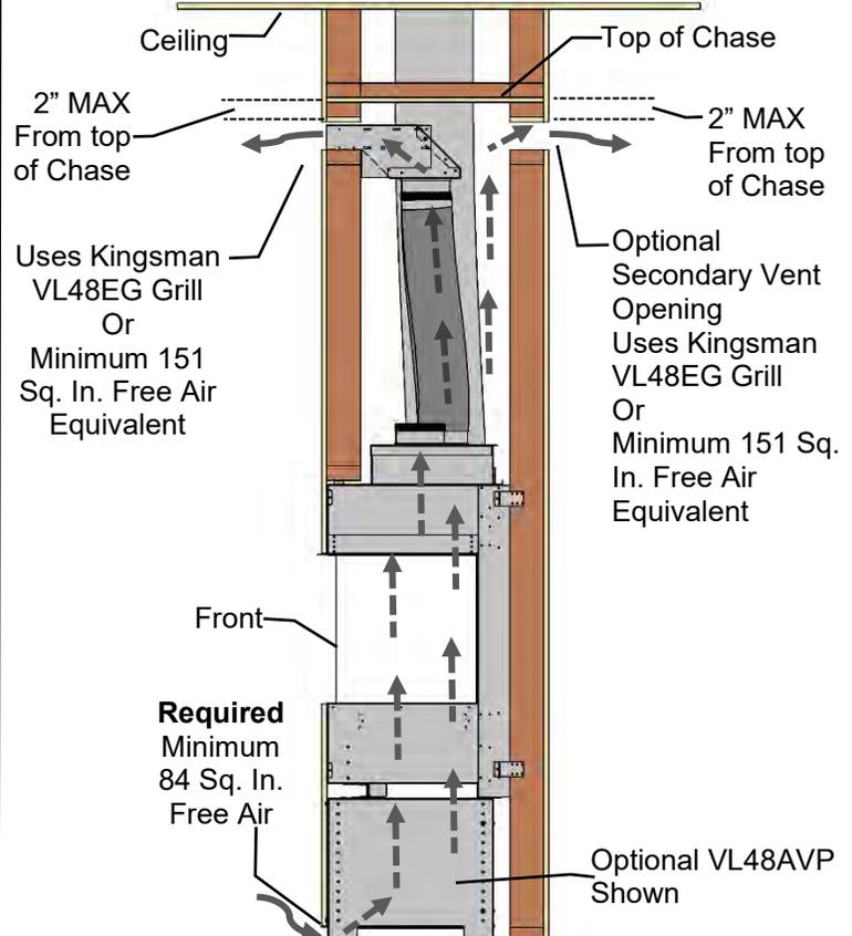
**Secondary Vent Opening Must Be In the Same Pressure Zone (Room / Area)**
