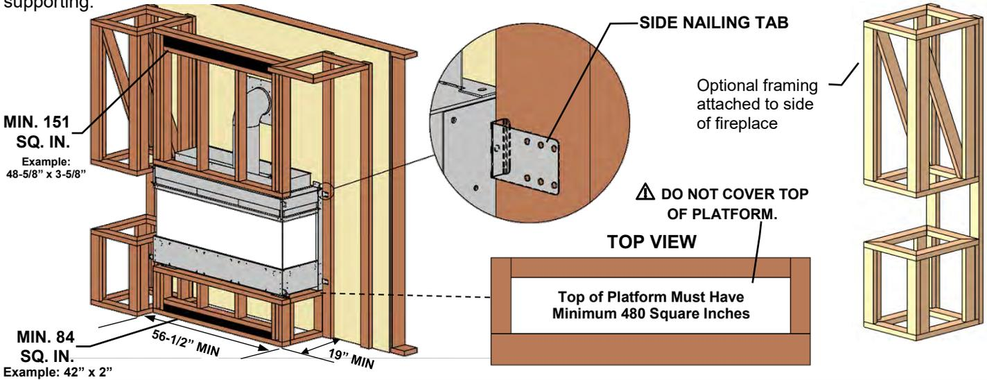
**OPTION B: Framing Attached to Top of Fireplace-** For cantilevered chase. Framing must be self-supporting.
