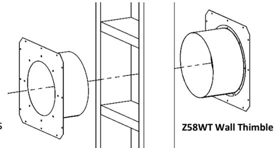
**Note: Vent Termination must not be recessed into wall or siding.**
