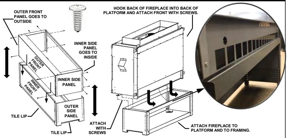
A Platform Base has air opening requirements that must be met.
