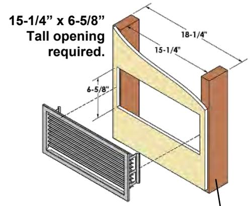
Vertical Studs are required for Pressure Fit
