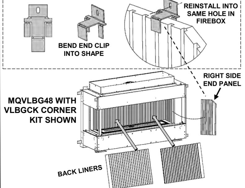
**STEP FOUR: Install Lower Liner Clips [x4].**
