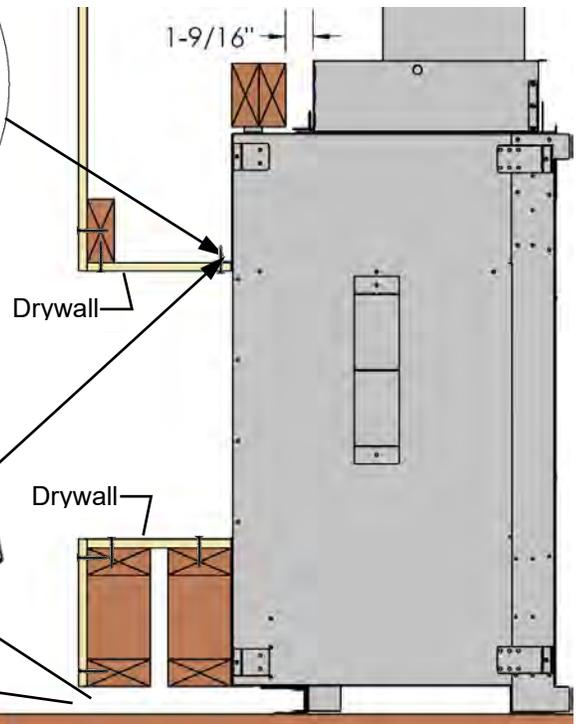
**NOTE:** If installing VL48S1BL or SS Surround: install Tile Lip using second hole from top, as shown. This will provide the required 5/8" clearance above opening.
