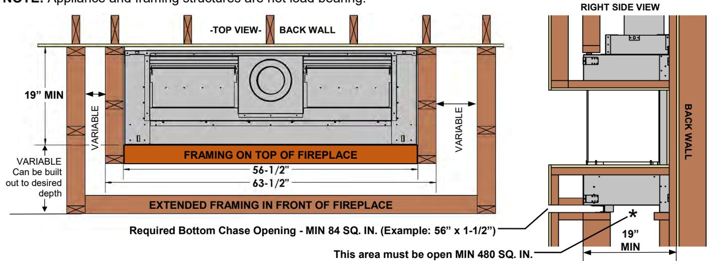
**OPTION B: Framing Attached to Top of Fireplace-** For cantilevered chase. Framing must be self-supporting.
