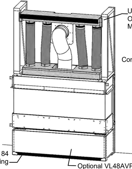
Connect only the two center pipes when venting to an optional secondary vent opening.
