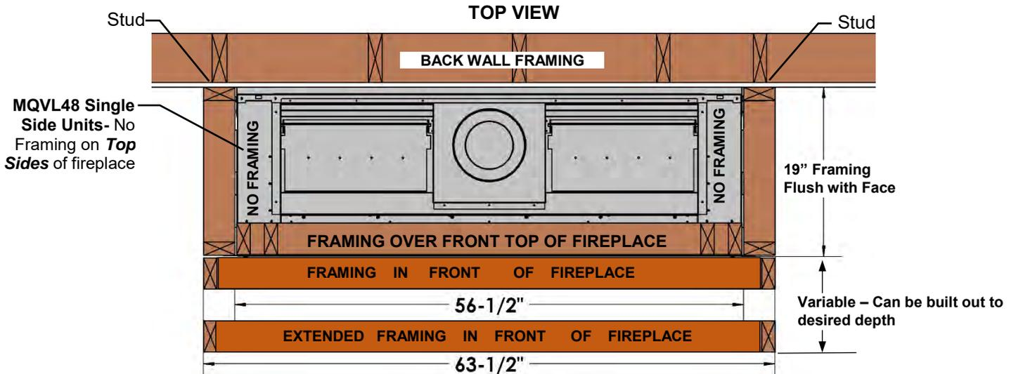
Appliance must be in place with venting connected before area above fireplace is framed in.
