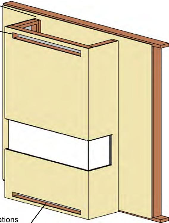
Lower Vent Slot (MIN **84 Sq. In.**) is REQUIRED for ALL Installations
