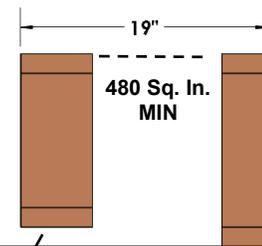
Opening must not be blocked by floor covering.
