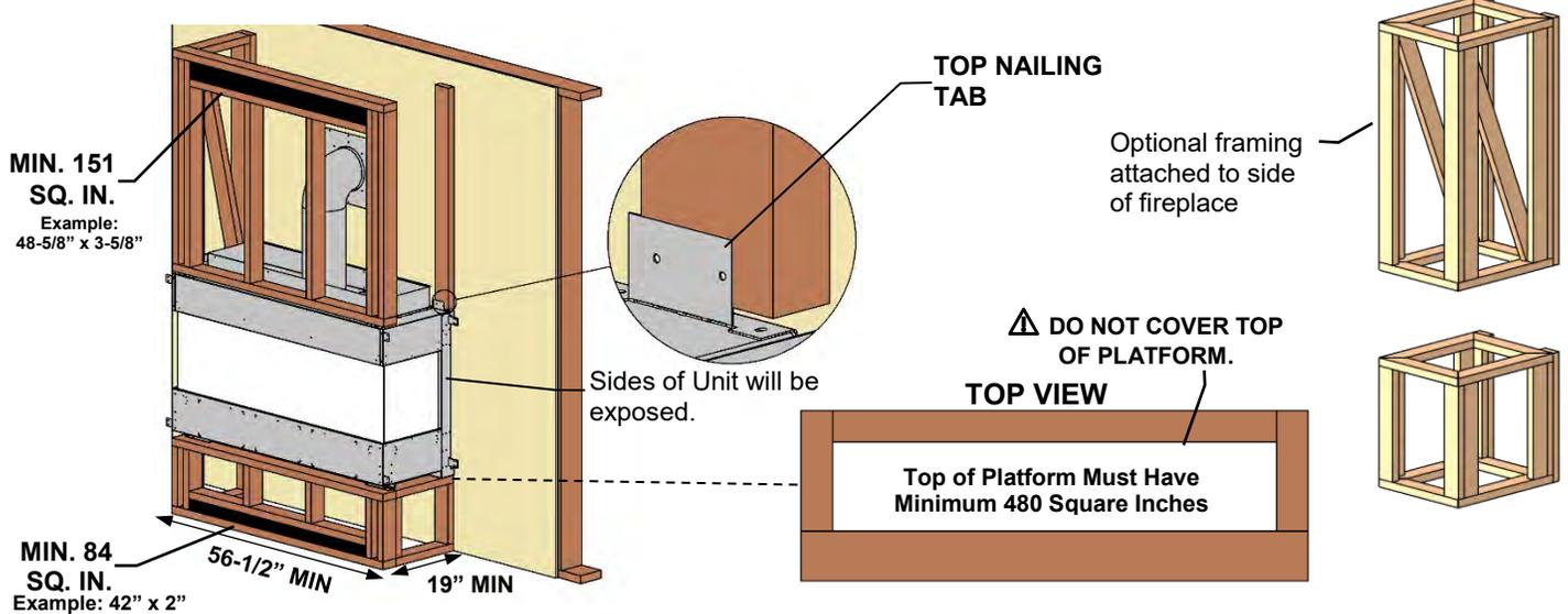
**OPTION C: Framing Attached to Back of Fireplace-** For cantilevered chase. Framing must be self-supporting.
