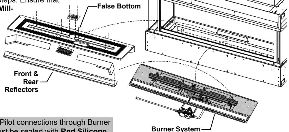
**NOTE:** Pilot connections through Burner Pan must be sealed with **Red Silicone**.
