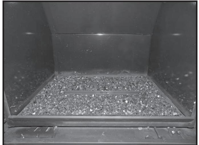
Figure 90: Crushed glass media in burner tray.
