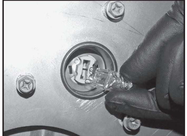
Figure 111: Replacing bulb.
