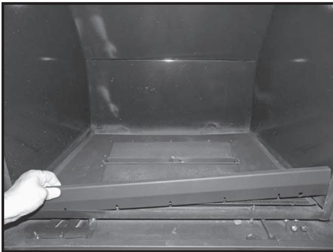
Figure 89: Inserting front trim piece.
