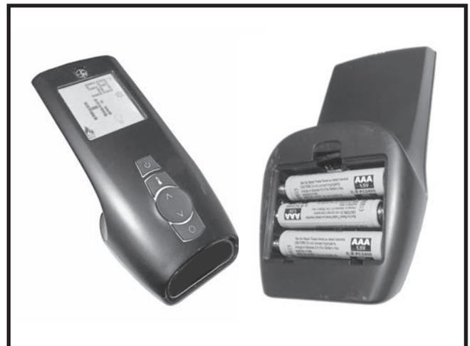
Figure 107: SIT remote handset and battery holder.
