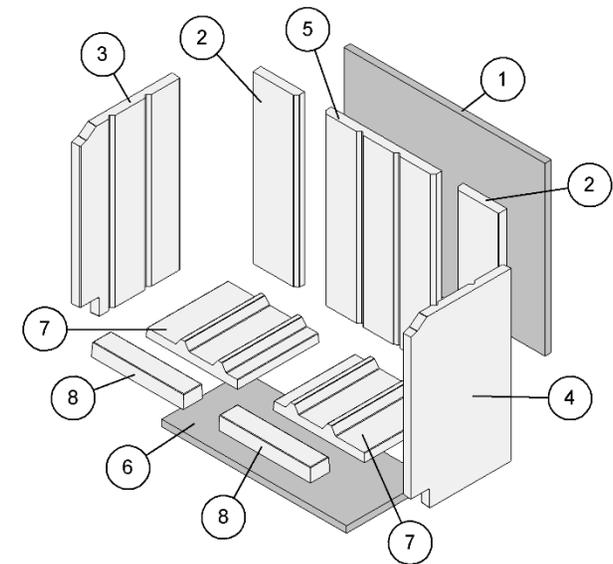
**Figure 4 Refractory Bricks and Insulation Panels**
