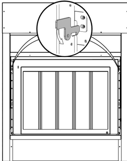
3. Ensuring the glass door is disengaged, pull the top of the door frame down and outwards to open in maintenance mode.
