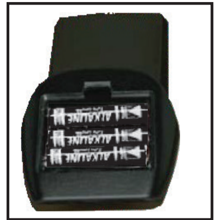
Figure 6: Proflame 2 remote battery compartment.
