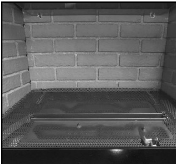
Figure 52: Burner with empty burner tray.
