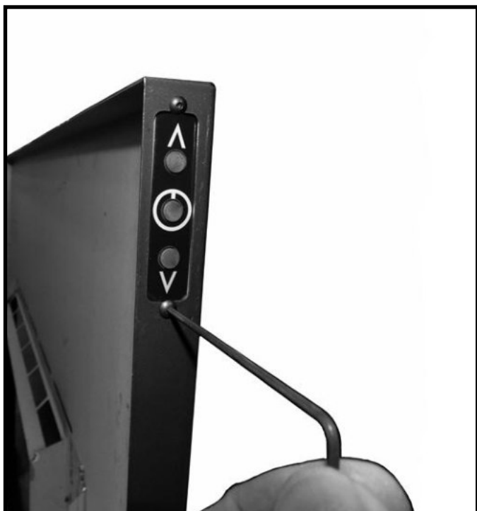
Figure 87: Attaching switch to backing plate.
