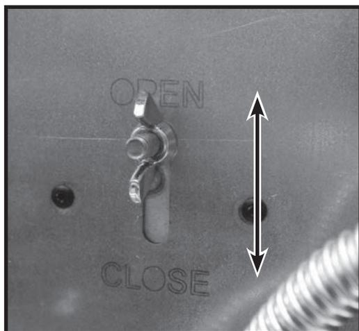
Figure 69: Venturi adjustment.
