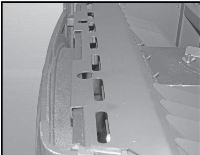
Figure 61: Screen holder in correct position.
