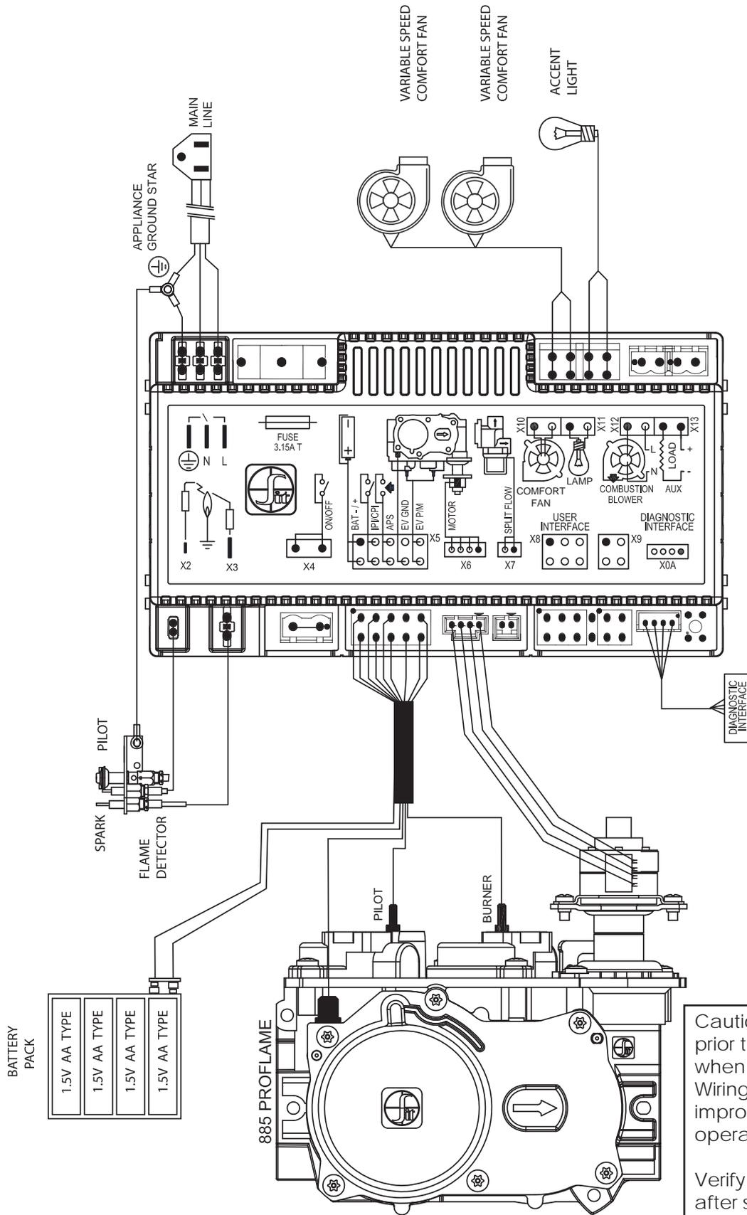
Caution: Label all wires prior to disconnection when servicing controls. Wiring errors can cause improper and dangerous operation.
