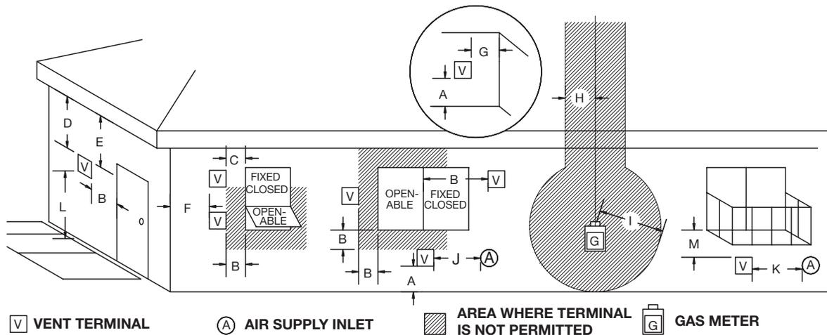
Figure 24: Minimum clearances to vents.
